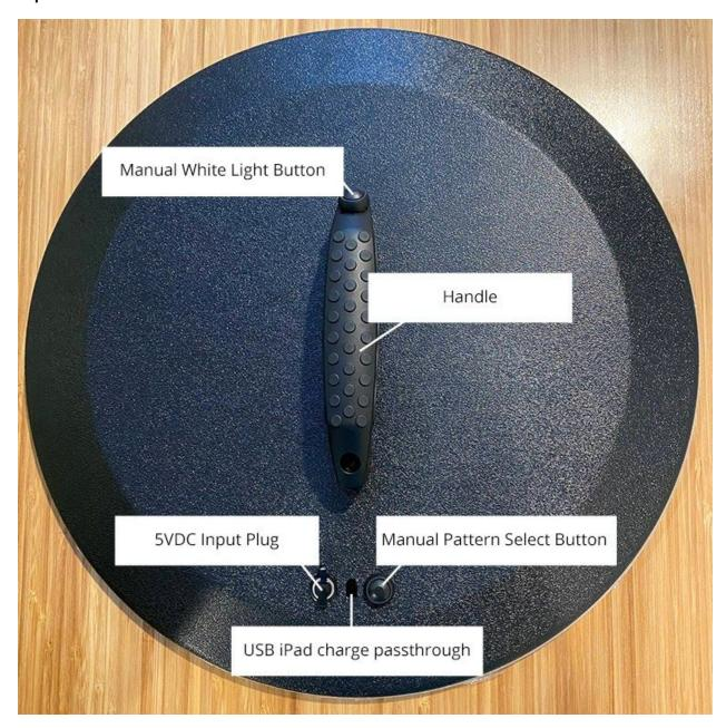
Manual White Light Button - used to manually switch all LEDs to white.
